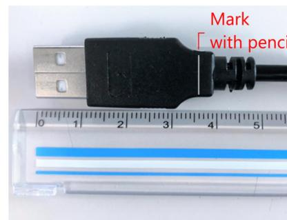
4. Turn white substrate inside connector up, Plug the connector into the holder to the
